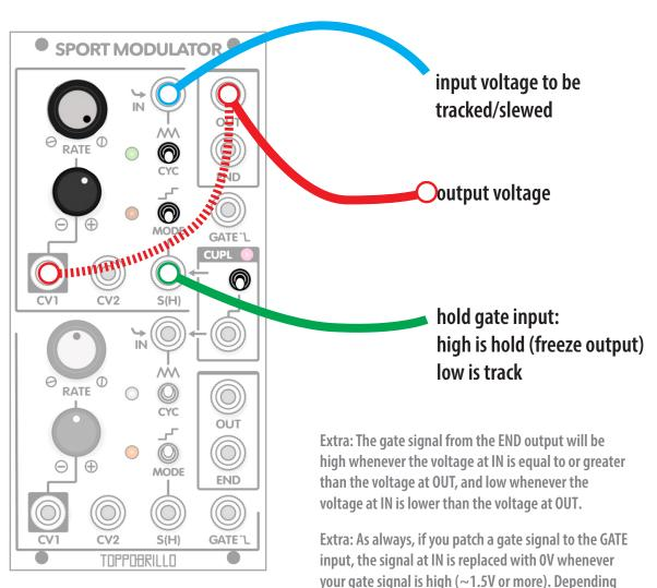
on RATE, this feature can be used creatively to nullify or distort the incoming signal (subject to RATE). Experiment.
