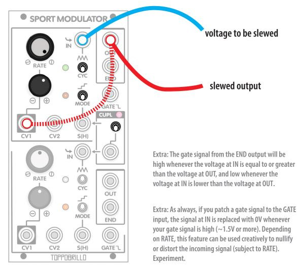
Set RATE high (fast) to pass incoming signal unaffected (no slewing). Set RATE lower (slow) to slew (smooth it out).
