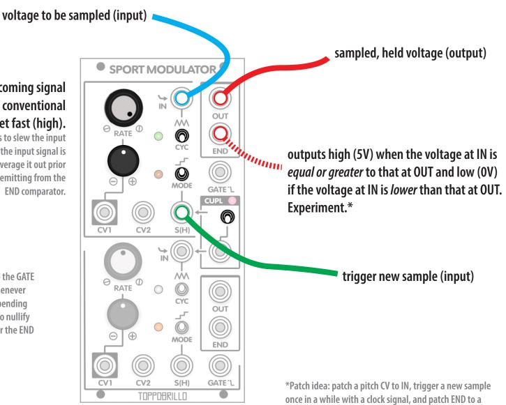
\*Patch idea: patch a pitch CV to IN, trigger a new sample once in a while with a clock signal, and patch END to a VCA controlling an effects send. The VCA will now close whenever the pitch at IN drops below the currently-sampled pitch.
