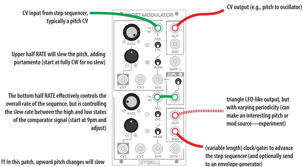
the progression of the sequence, and downward pitch changes will speed it up. It is crucial to experiment with the sequence while it is playing.
